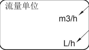
The display shows '流量单位' at the top, 'm3/h' in the middle, and 'L/h' at the bottom. An arrow points from 'm3/h' to the label '当前值' (Current value) and another arrow points from 'L/h' to the label '更改值' (Change value). |
